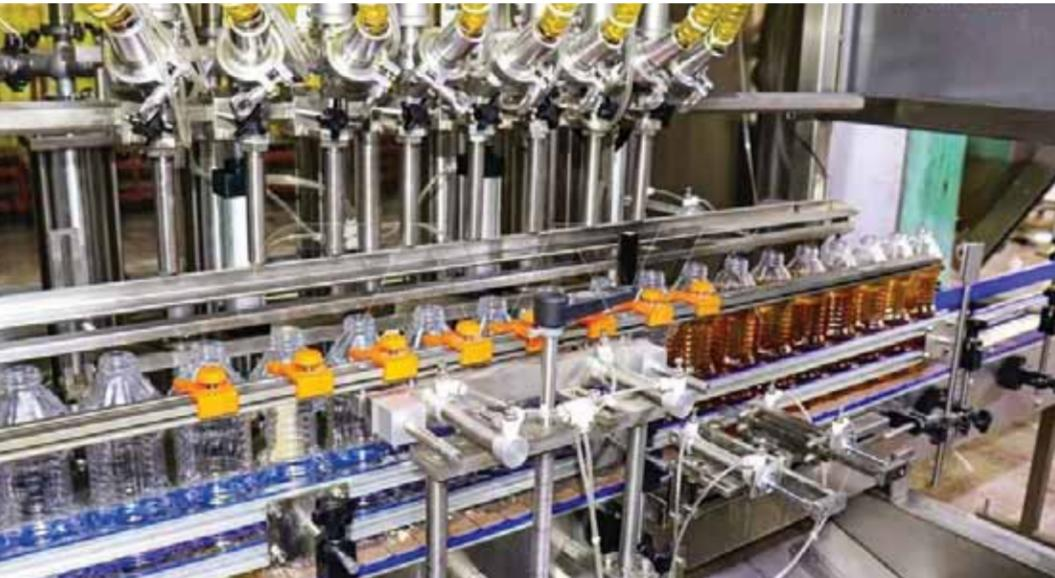
The image shows a complex industrial bottling or packaging line. Numerous clear plastic bottles are moving along a blue conveyor belt. Above the conveyor, a series of stainless steel dispensing arms are positioned, each equipped with a nozzle to fill the bottles with a dark liquid. The machinery is highly automated, with various pipes, valves, and sensors visible. The background is a bright, well-lit industrial interior.
